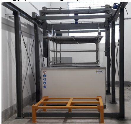
System wannowy do strippingu
